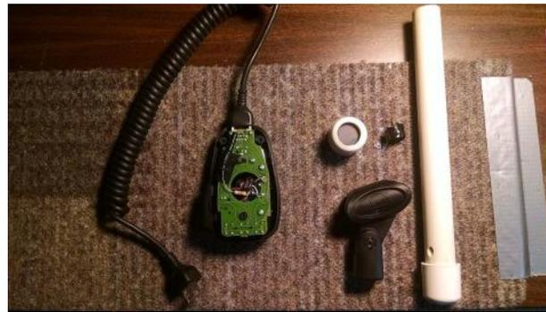
On this second picture, you can see the MH-31 after the electret element was installed.
