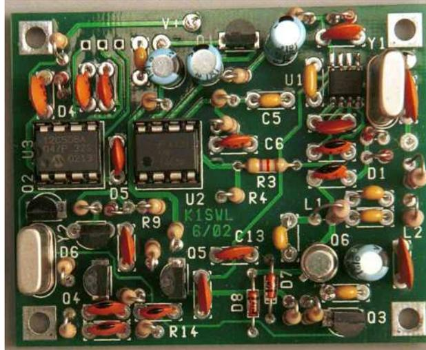
The Rockmite is a CW only transceiver with a built-in keyer, or provision for use with a straight key. Nice feature. Output power is only  $\frac{1}{2}$  watt with a 12V supply and can be run on as little as a 9V battery at a reduced power. For more detail, here is their web site.
