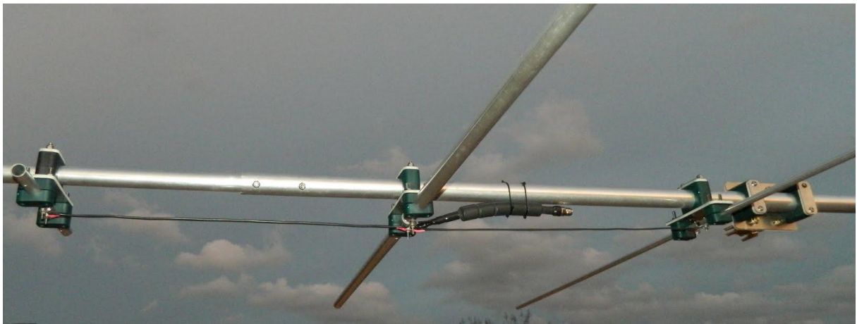
Figure 23 – Phasing lines flank element #5, the 20 Meter element, which is where the 1:1 balun attaches. This photo shows a thick, black W2DU style bead balun installed via tie-wraps to the boom above the phasing lines. Coaxial choke baluns can hang below the feedpoint.
