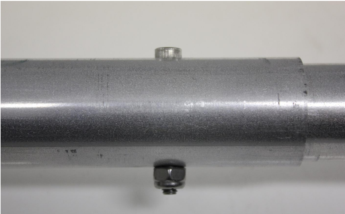
Figure 9 – Nylon lock nut placed on the opposite end. The socket cap head faces upward when installed on the antenna, the nylon nut faces down
