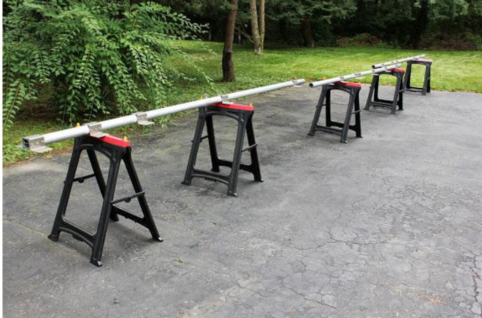
Figure 3 - Lay boom sections out on sturdy saw horses in order.
