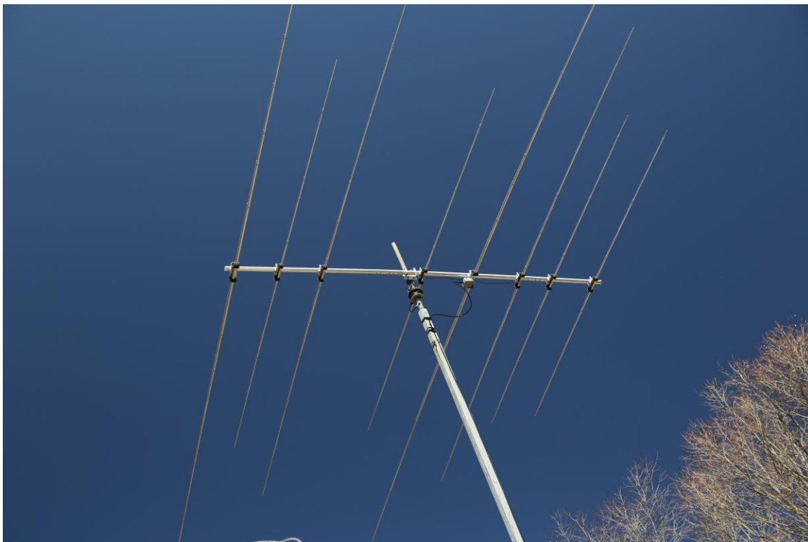
Figure 26 – Completed TX38-100 installed on a US Tower 40 foot mast.
