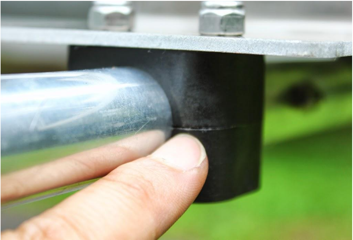
Figure 14 – Tighten the nylon clamp evenly. Alternate between each bolt to avoid galling. The gap between the blocks should just close when the torque is correct. Do not continue to add additional torque after the gap closes.
