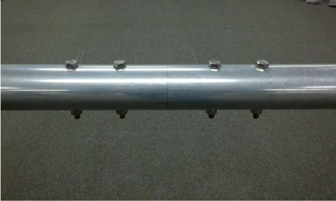
Figure 4 - Boom splice installed. The hex head should face up and the nylon lock nuts should face down.
