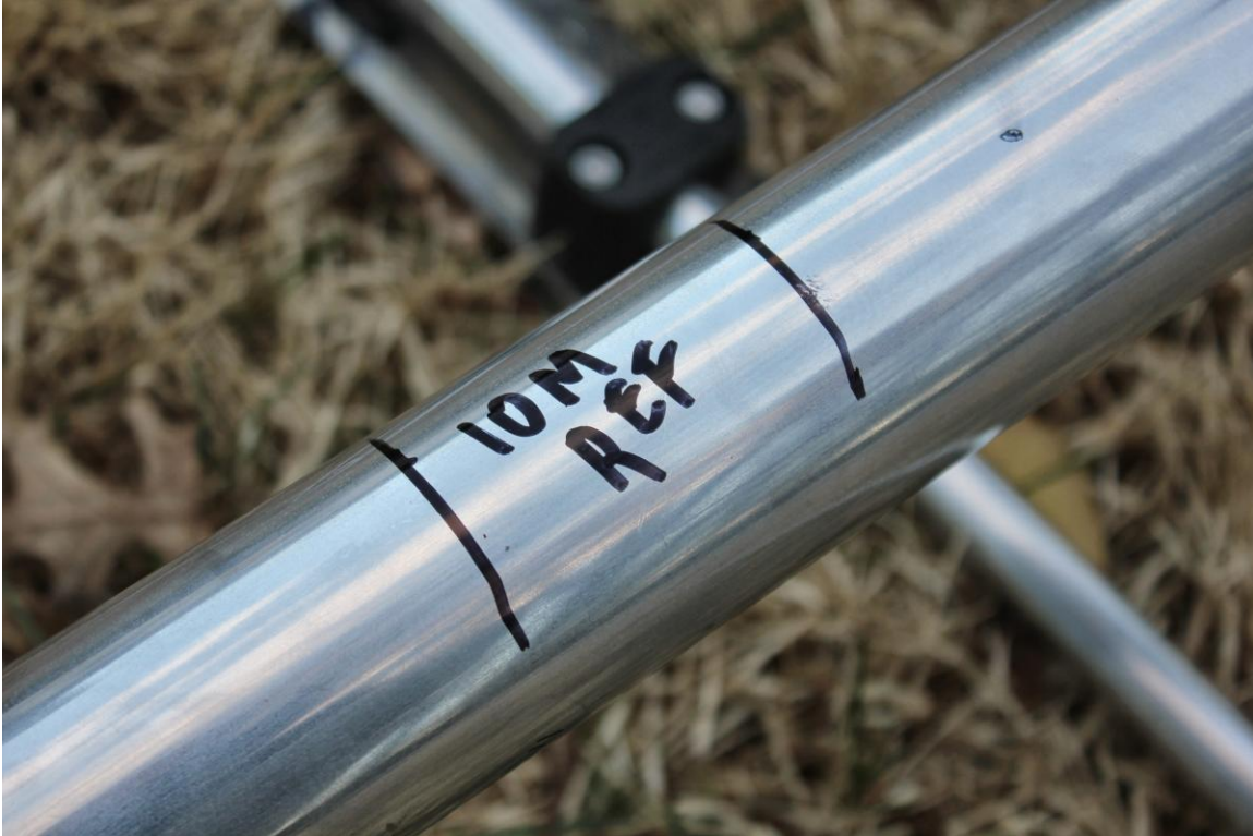
Figure 18 – You may wish to mark the boom with the approximate position of each element plate, so that when you are initially mounting element plates that you can quickly place them onto the boom
